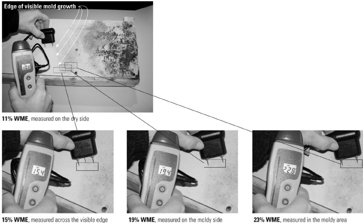
**Figure 5** Gypsum board moisture content often varies widely across short distances. Consequently, it is important to note the exact locations from which measurements are taken. Also, moisture readings between instruments from different manufacturers seldom correlate. For consistent interpretation of mold and moisture risk, record the instrument make and model number and which of its several moisture scales was used to take the readings.
