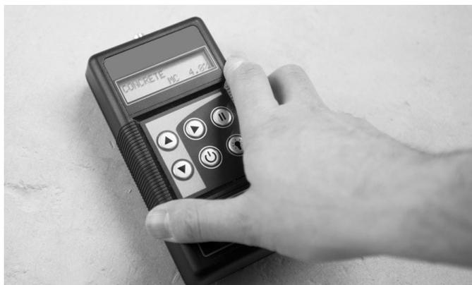
**Figure 7** Capacitance instrument to estimate moisture content in concrete and masonry block. Although not considered conclusive, capacitance moisture meters are often used to approximate moisture content. The technique does not require drilling holes or a 72 h waiting period. It can be used to take many measurements quickly, allowing construction of a visual moisture map, as shown in Figure 8.
